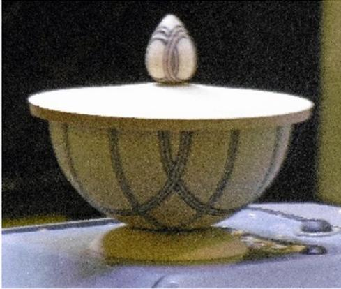
Carlyn sawed through the spigot to release the lid. A jam chuck was turned in a scrap piece and the lid reversed onto it. The top was finished by making the slope slightly concave and the stub, from where it was cut off, was turned down so that the small finial could be fitted.
